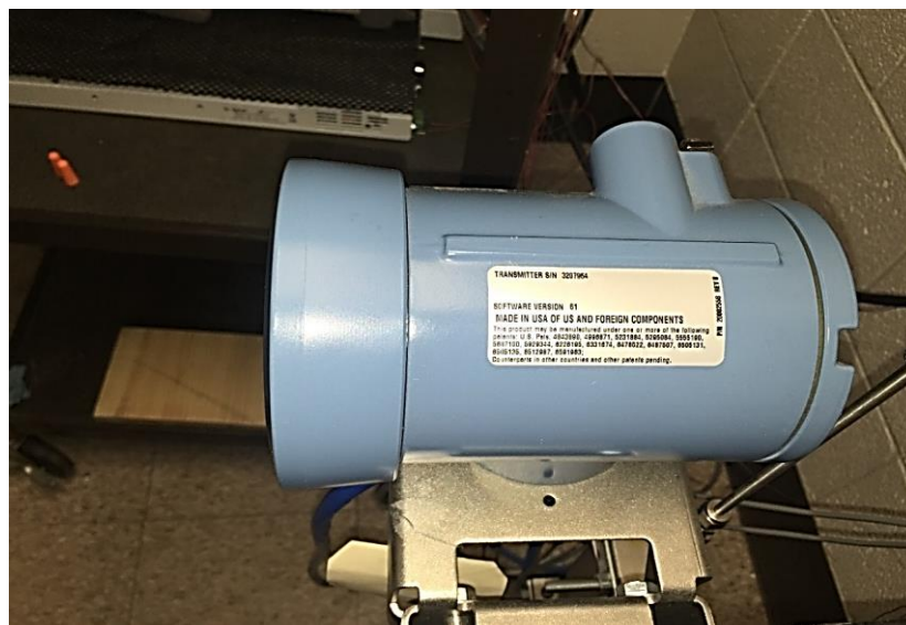
Figure 8 Pressure transmitter in-use position
