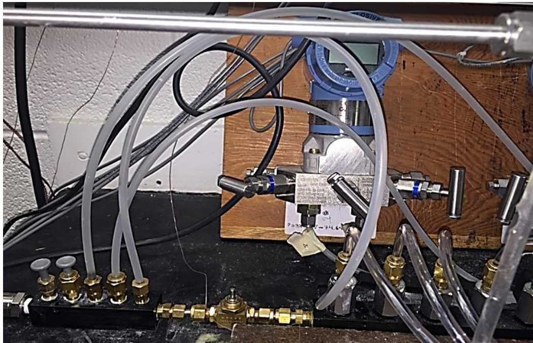
Figure 7. Pressure tubes-transducer connection
